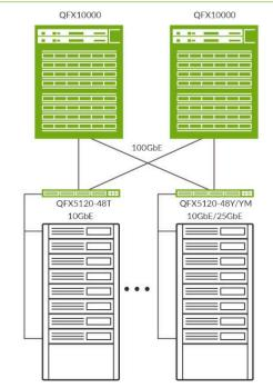
Figure 2: QFX5120-48T and QFX5120-48Y/48YM as leaf and QFX10000 as spine switches
